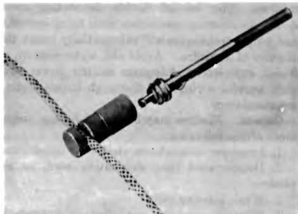
Figure 40—Priming with Other Firing Devices Coupled to Initiator.
