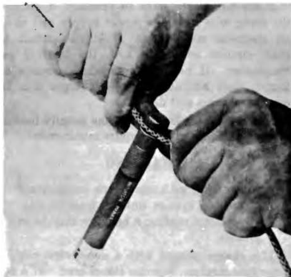
Figure 38—Attaching Initiator to Detonating Cord.
