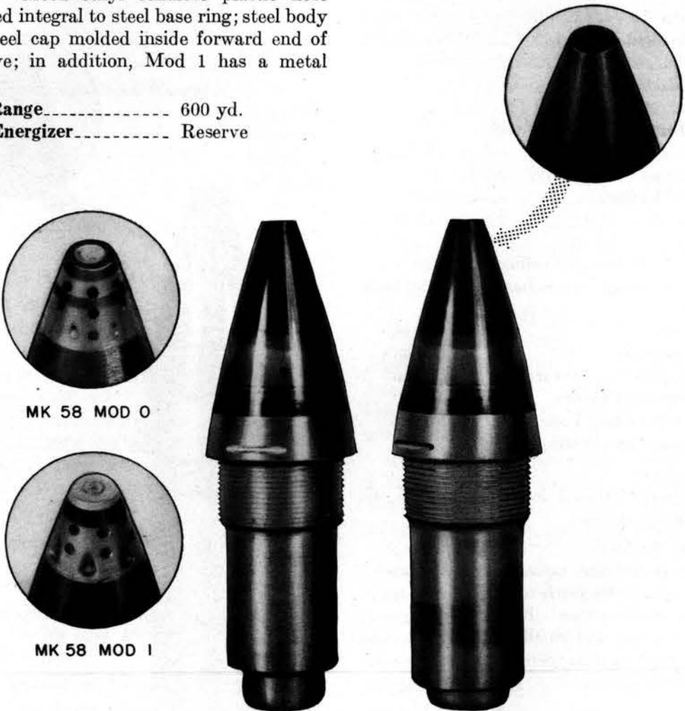
MK 58 MOD 2 MK 58 MODS 3 & 4 Figure 12. VT Fuze Mk 58.
