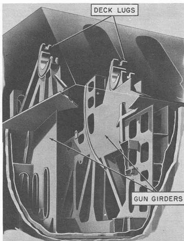
FIGURE 7H4.—8"/55 RF gun and turret. Gun-supporting construction.
