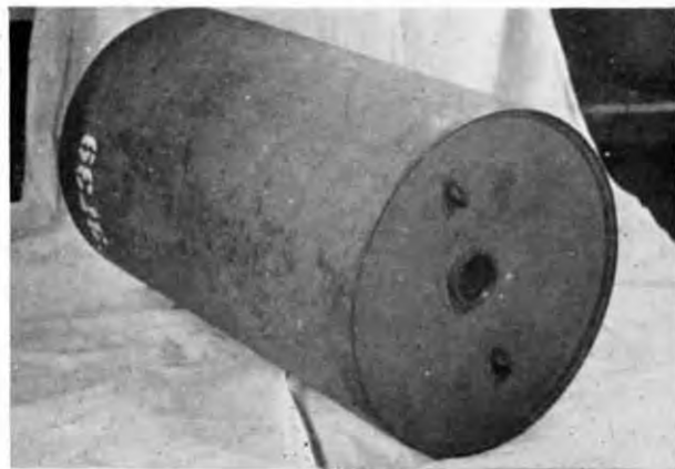
Figure 28—Two views of the Type 95 depth charge. Note the bolted end plate.
