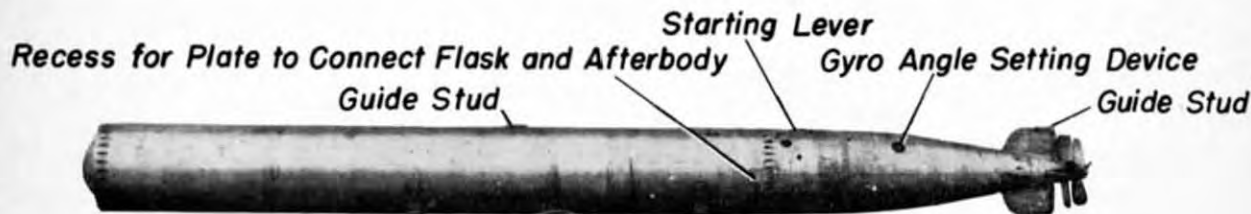
Figure 30—Type 6th year torpedo with warhead removed.
