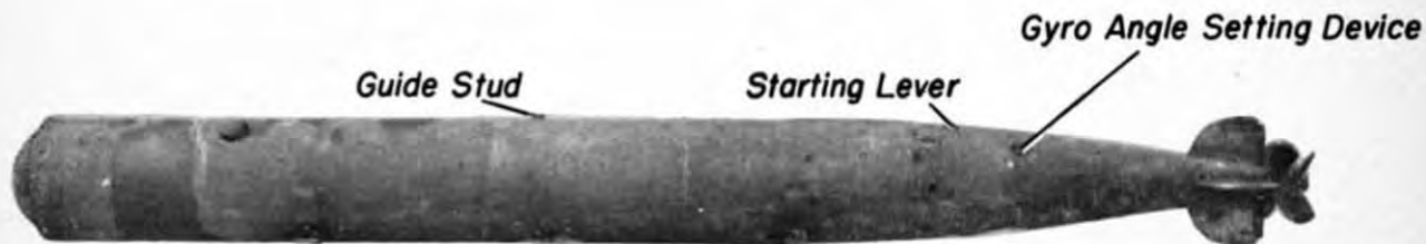
Figure 29—Type 44 torpedo with warhead removed.
