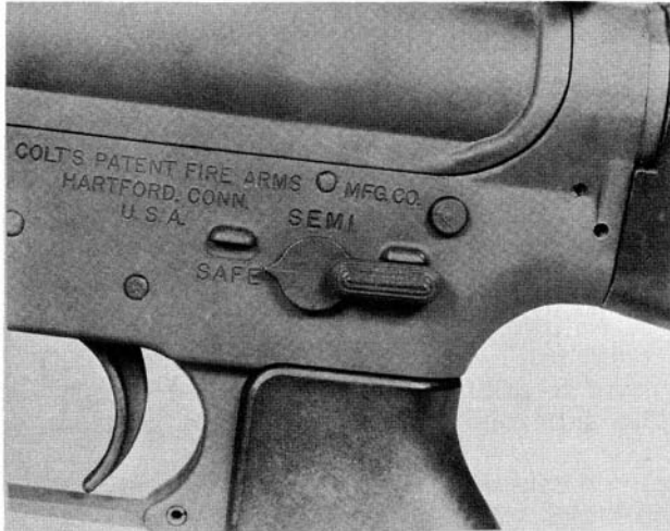
Figure 11-21. — Selector lever pointing to SAFE.
