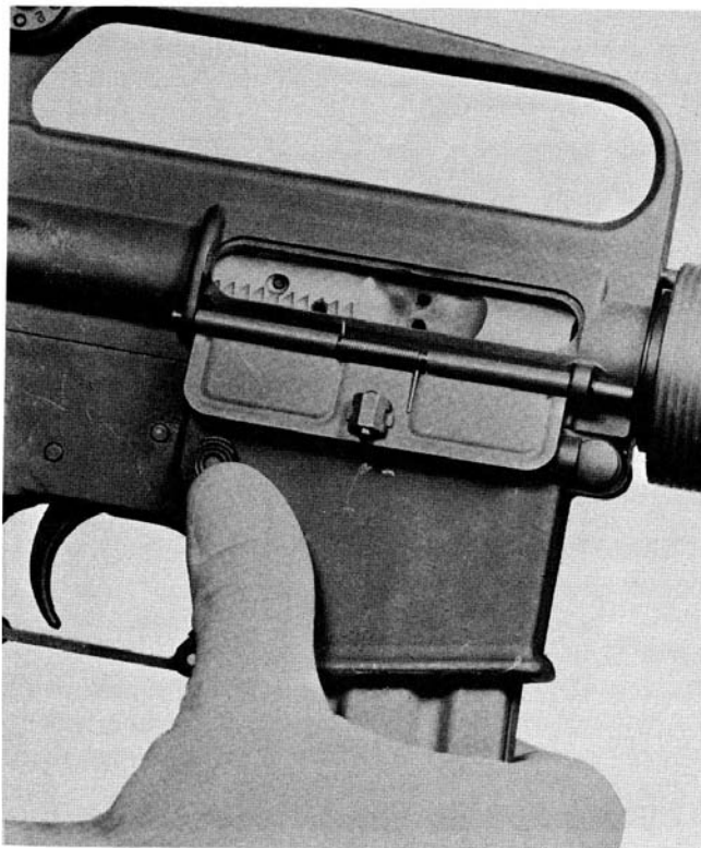
Figure 11-22. — Removing the magazine.
