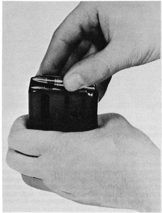
29,360 Figure 11-35. — Loading cartridges into magazine.
