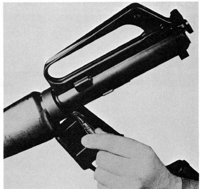
29,352 Figure 11-27. — Pressing out receiver pivot pin.
