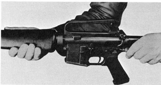
29,350 Figure 11-25. — Pressing takedown pin to the right.
