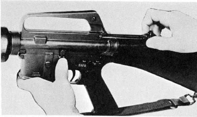
29,349 Figure 11-24. — Locking the bolt open.
