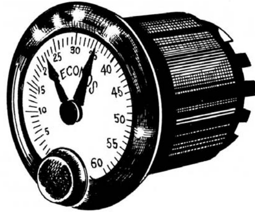
Figure 9-22. — Automatic reset timing relay.
