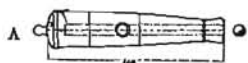
A.—The 42-pounder of 1812. Length, 10 feet; weight, 4 tons; charge, 10 pounds; projectile, 42 pounds; muzzle energy, 800 foot tons.
