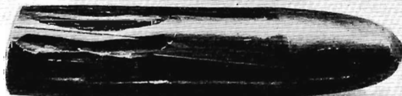
FIG. 267.—Effects of Erosion on Bullets.
