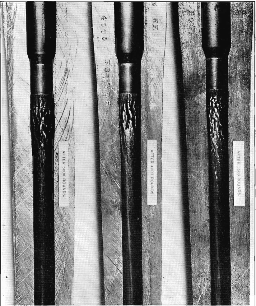
FIG. 266.—Erosion in Rifle Barrels.
